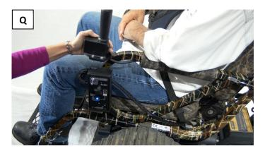
Loosen the star knob on the AutoLeveler, rotate the AutoLeveler until both A and B motor lights go out (R-T), then retighten the knob.
