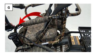
Follow the chair's manual tilt switch cable to the back of the chair and under the seat (H-J). You can follow it from the tilt switch, along the arm rest, down the frame, to the back and under the seat.
