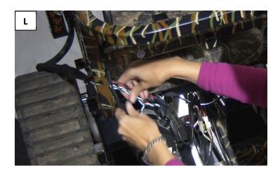
Unhook the connector on the red & black cable by pressing the release latch (**M**). Hook together the connectors from the AutoLeveler's red & black cable to the chair's red & black cable, matching male to female and female to male (**N**). (NOTE: a spark or pop when connecting the cables is normal and harmless.) Repeat this process for the green & white cables (**O**). Coil the cable in a place where it won't be pinched by the chair tilting or caught in the wheels.
